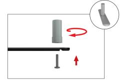
**Step 5:** Push banner stand frame onto posts of flat base or optional feet. Press evenly on both sides to make easier for the frame to go on.
