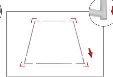
**Step 5:** Assemble post (75) into base plate or optional feet with screw by hand turning post and tightening into place.
